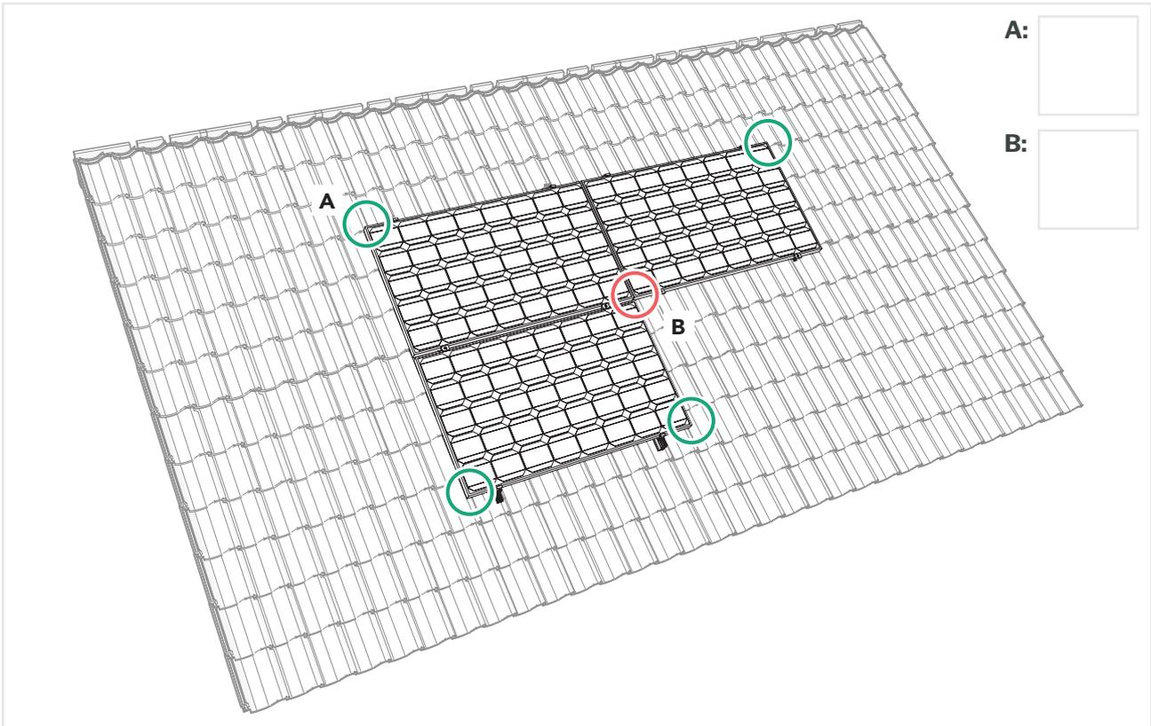
**2** Measure the maximum distance from the edge of the panel to the roof surface (**X**).
